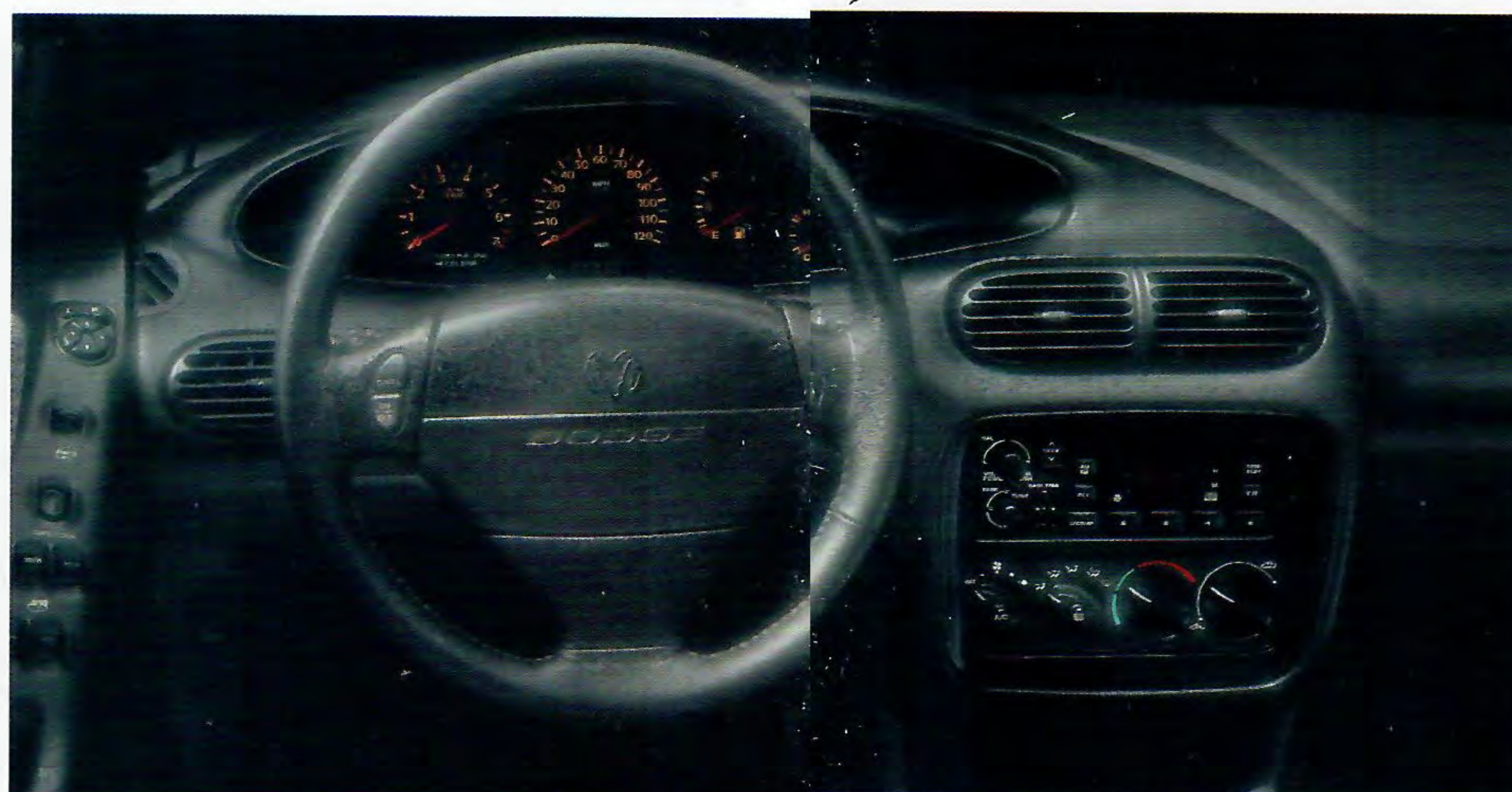
Stratus' ergonomic instrument panel design (above) provides a clear view of all gauges (tachometer, speedometer, fuel and temperature) through the steering wheel.
