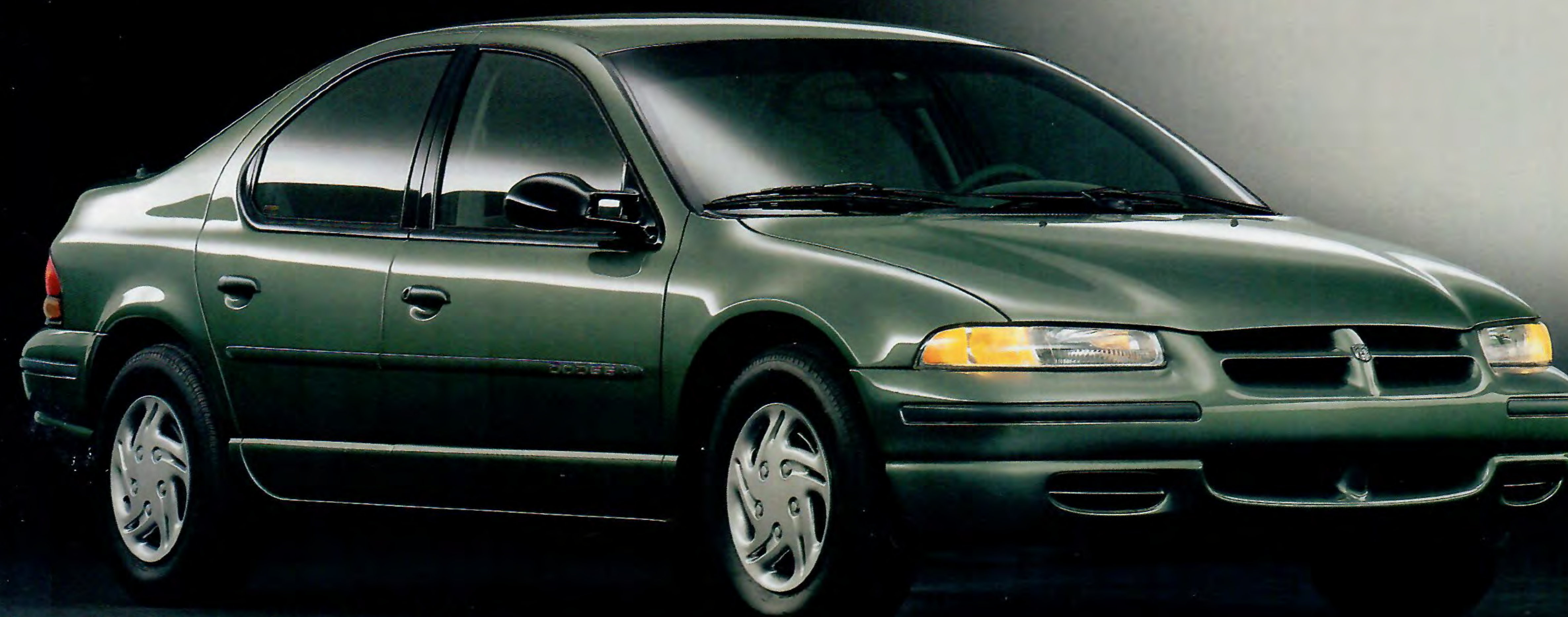
Stratus, shown in Medium Fern, with standard 14-inch wheel covers and P195/70R14 tires. All tires and wheels ride flush with Stratus fenders for a "full wheel well" look.
